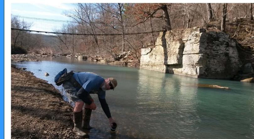
Figure 7 - Water samples were taken at each location and measurements of pH, electrical conductivity, and temperature were made. GPS readings were also made.
